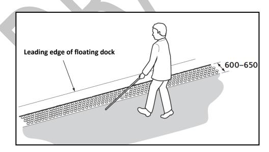
Figure 22: Detectable Hazard Indicator Surface (CAN/CSA-B651)
