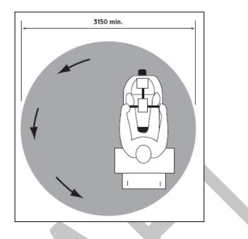
Figure 8: Turning area (in mm) for a person using a large scooter (CAN/CSA-B651)
