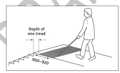
Figure 25: Detectable Warning Indicator Surface (CAN/CSA-B651)
