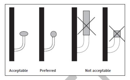
Figure 21: Handrail Shapes (CAN/CSA-B651)
