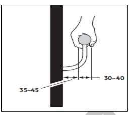
Figure 18: Handrails (CAN/CSA-B651)
