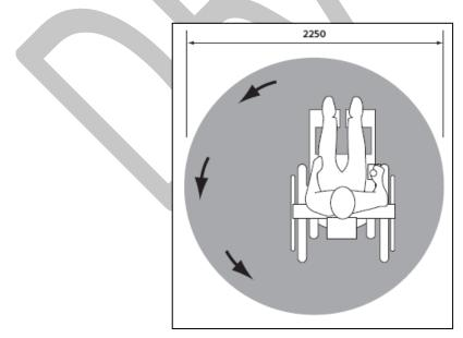
Figure 7: Turning area (in mm) for a person using a power wheelchair (CAN/CSA-B651)
