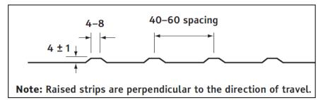
Figure 26: Detectable Warning Indicator Surface Configuration (CAN/CSA-B651)
