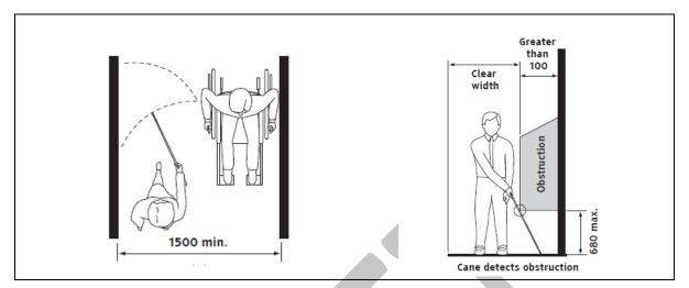
Figure 12: Detection space (in mm) for persons using a long white cane (CAN/CSA-B651)
