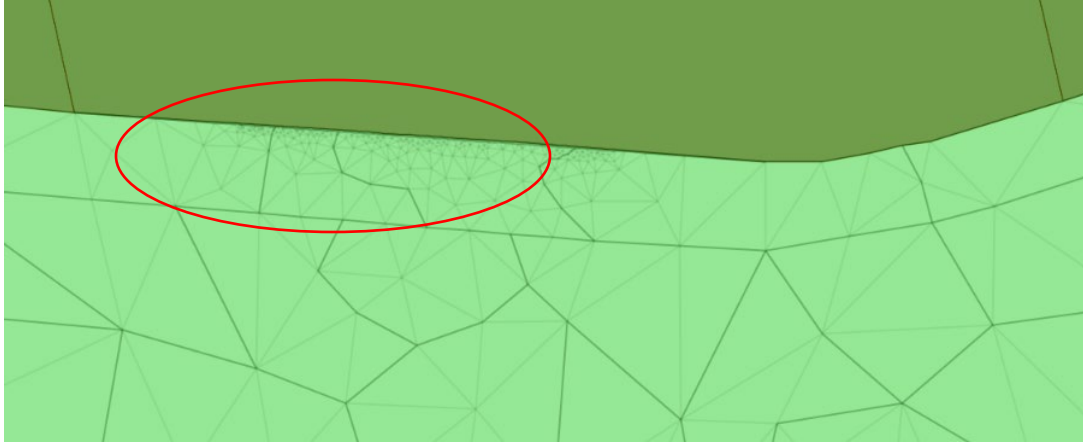
Figure 6-7 Example of Excessive Triangulation of 2D Mesh
