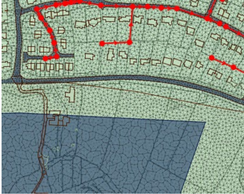
Figure 6-8 Mesh Zones (in blue) to decrease the resolution of the 2D mesh and to represent roads
