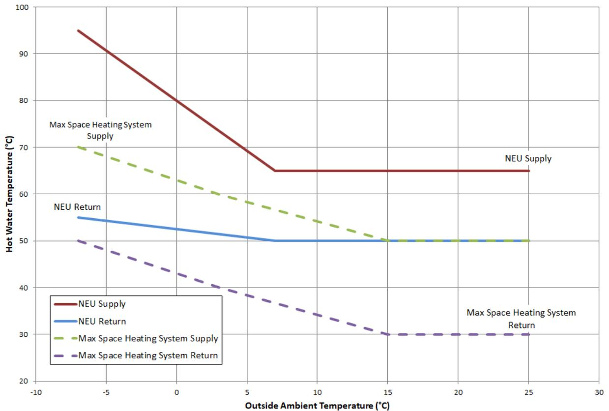
**Figure 4: NEU System and Building Heating System Temperatures**
