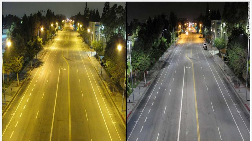
LEDs produce a whiter light that renders colours more accurately and improves colour contrast. Lights that render colours more accurately have a higher **colour rendering index (CRI)** rating.
