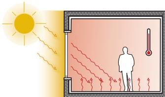
*In a room without thermal massing, heat from the sun is reflected into the room causing uncomfortable warmer temperatures*
