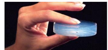
□ Many aerogels are translucent – and can be used to insulate windows and skylights or create translucent walls.
