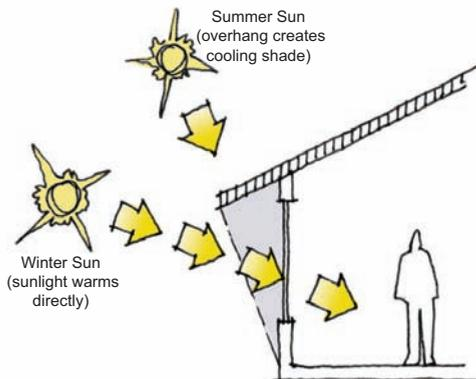
*Because the winter sun is at a lower angle, sun can travel directly into the building warming it during the cool months. The high summer sun is blocked by the overhang creating a cooling shade.*
