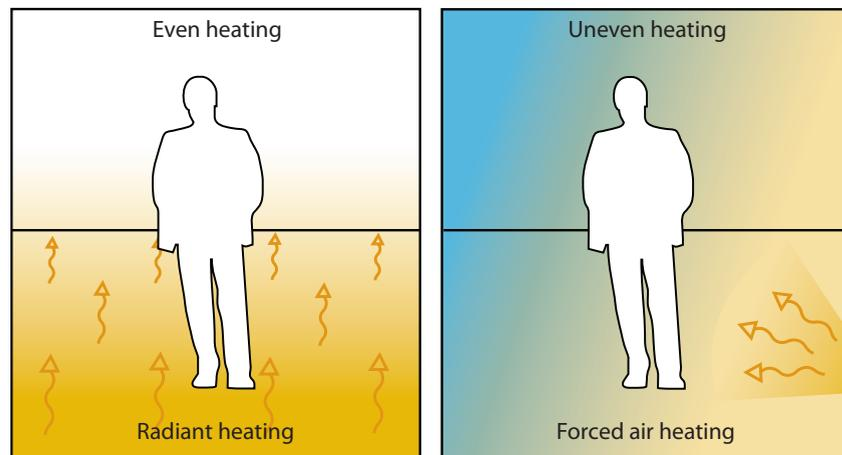
Radiant energy can be beneficial – this type of energy is emitted from a heat source and is different from tradition convection heating. This type of heating can penetrate all objects in its path and rather than heating the air, directly heats all objects in its path, including people.
