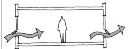
Cross ventilation occurs between windows on different exterior wall elevations. Patio and screen doors are also effective for cross ventilation. In areas that experience unwanted solar gain, operable clerestory windows or ceiling/roof space vents can aid with ventilation and cooling (see Section 8.3).
