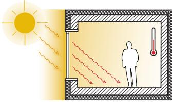
*Sun enters room and heat is absorbed into flooring keeping the room temperature comfortable*
