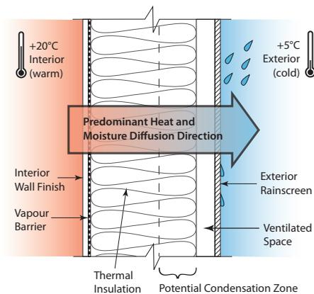
An air barrier system should be continuous around all components of the building, with special attention given to walls, roof and the lowest floor. There must be proper continuity at intersections, such as the connection between floors, the joints between walls and
