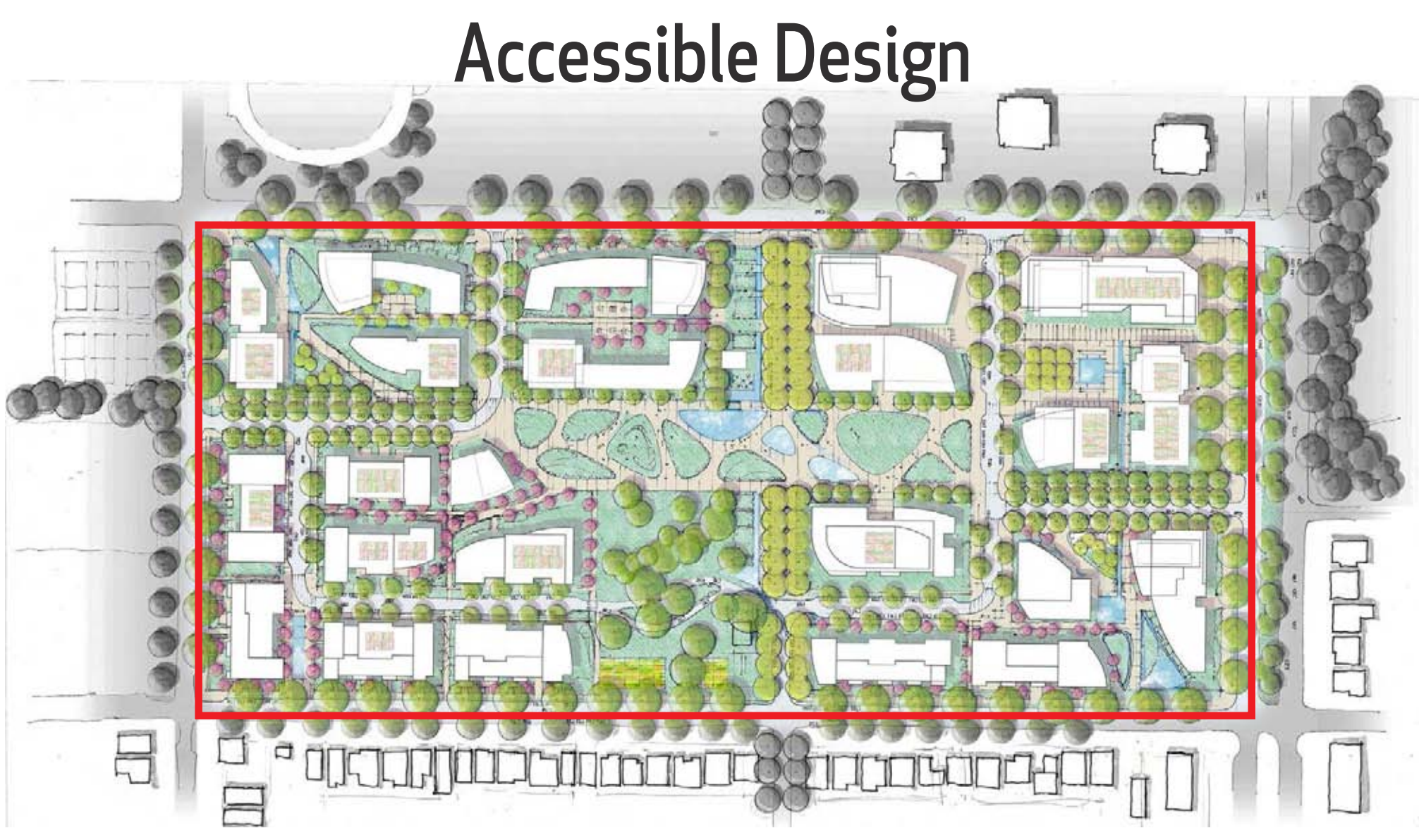
Accessible Design Detailed design throughout the site (buildings, linkages, and public spaces) will carefully consider accessibility and utilize a leading edge approach to accessibility design. Currently all connections are below the maximum 5% slope threshold for universal design.
