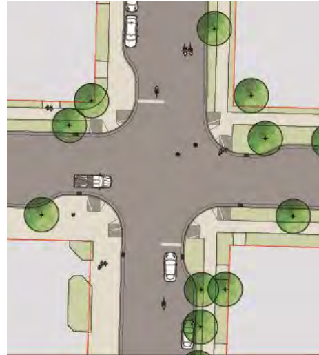
Diagram 2: Typical intersection design with curb bulges
