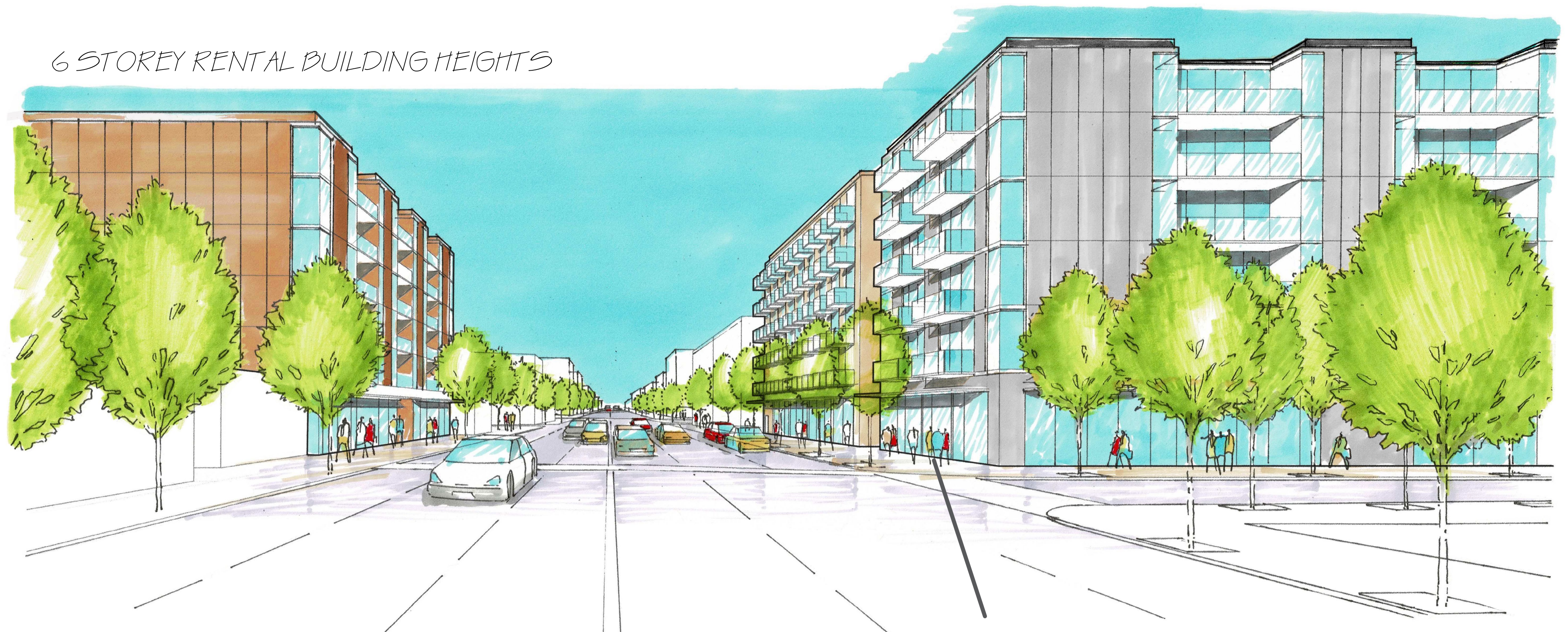
FRONT BUILDING SET-BACK FROM THE PROPERTY LINE AT GROUND-LEVEL FOR SIDEWALK WIDENING
