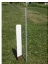
The most frequently used survey monument is the galvanized iron post. It is used to mark the boundaries of city lots, small holdings, mineral claims and rights-of-way.
