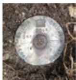
The capped post is used to mark the corners of district lots or sections. The capped post is also found along highways and other rights of way.
