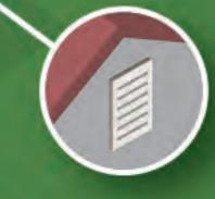
Add non-combustible 3 millimetre screens to external vents (except dryer vents).
