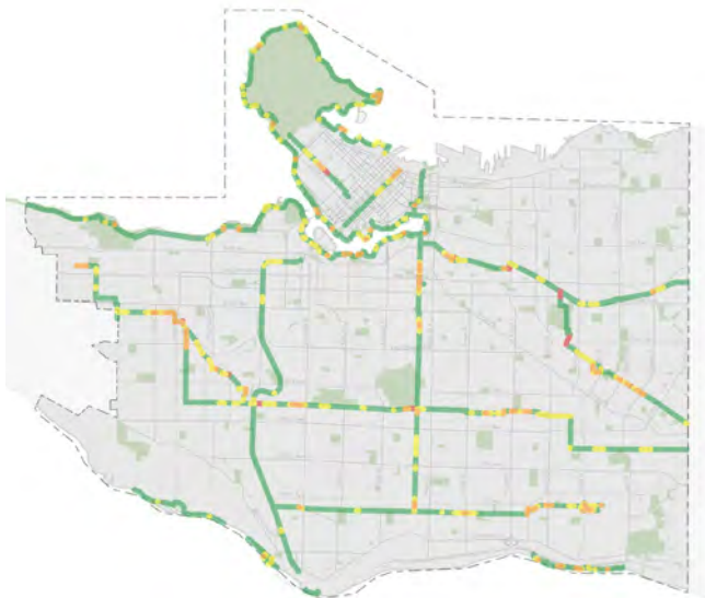
Figure 35. Existing Greenway Slope Analysis + Proposed Greenways — < 3% — 3 - 5% — 5 - 7% — > 7%
