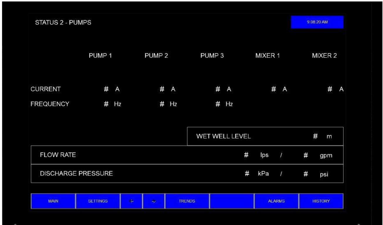
Figure 6: PLC HMI Screen #6 (Typical)
