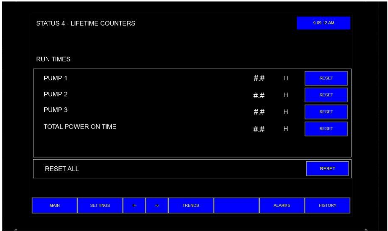
Figure 7: PLC HMI Screen #7 (Typical)
