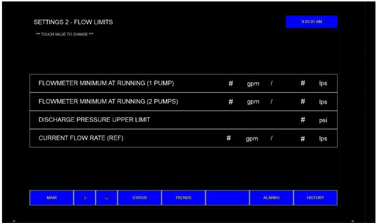
Figure 3: PLC HMI Screen #3 (Typical)
