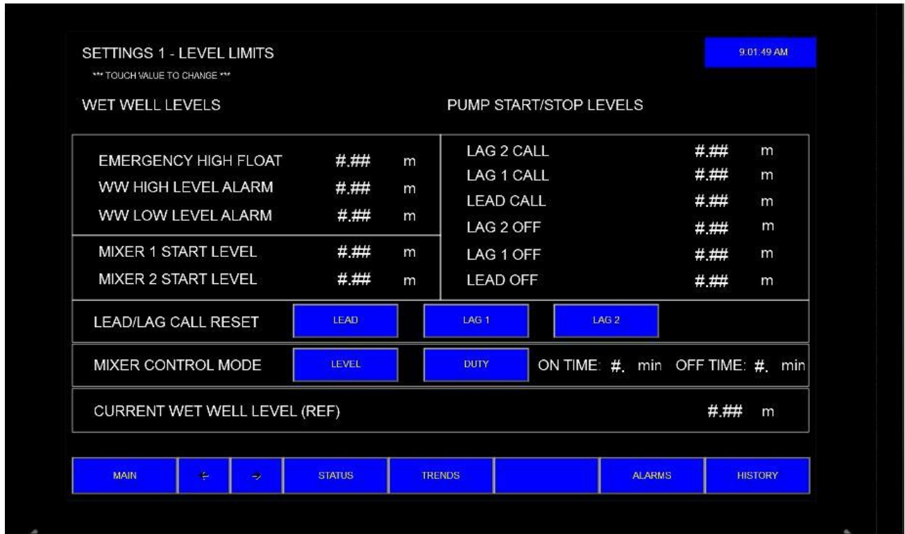
Figure 2: PLC HMI Screen #2 (Typical)
