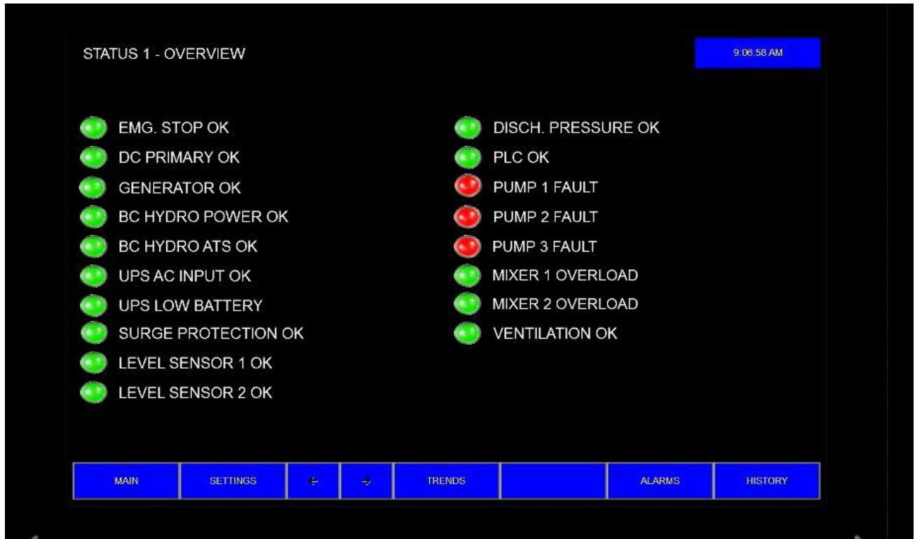
Figure 5: PLC HMI Screen #5 (Typical)
