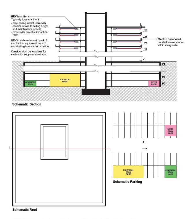
Electric baseboard heating with a centralized electrical resistance boiler for domestic hot water production and for the corridor ventilation system.
