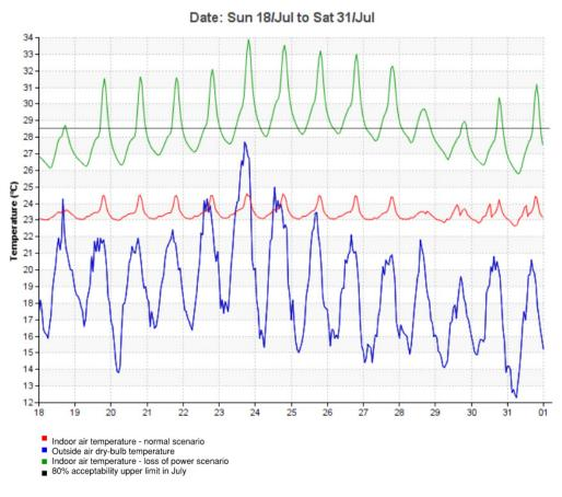
Figure 2.6: Indoor Air Temperature with Loss of Power Compared to the Normal Scenario for Zero Emission Option 3
