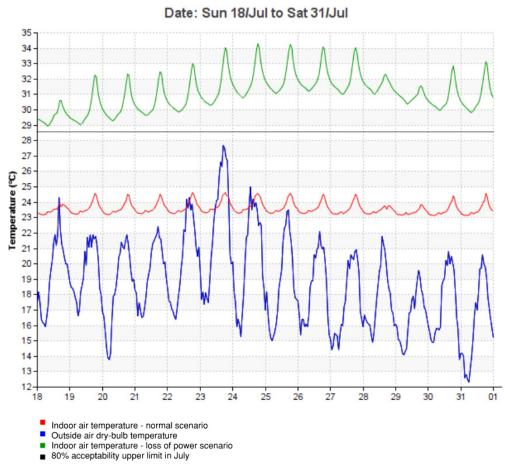
Figure 2.10: Indoor Air Temperature with Loss of Power Compared to the Normal Scenario for Zero Emission Option 3
