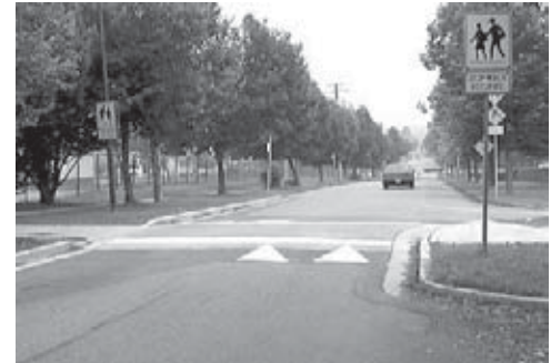
Raised Crosswalk: traffic calming to slow cars
